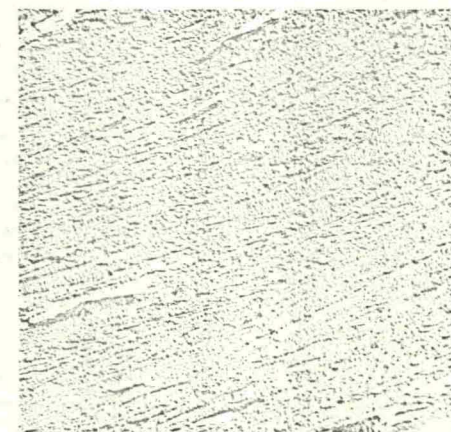
51 Carbon replica of solid-phase bond in Fig. 14. \times 1200 .
