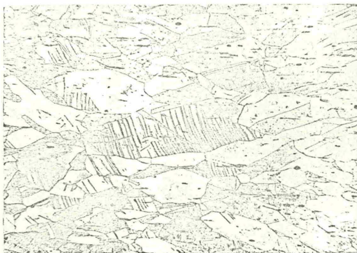
57 Mechanical twins in explosively welded copper. \times 200 .
