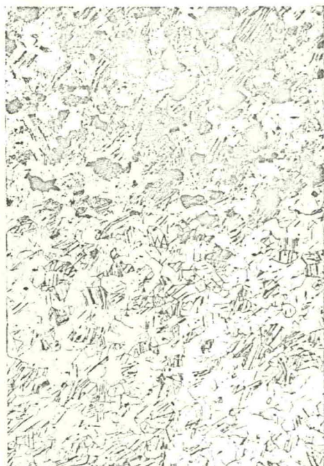
59 Shocked zone in iron. \times 80 .
